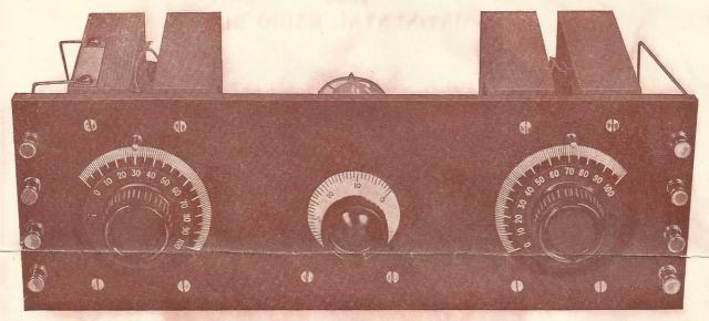
After the filament current is turned on (by the rheostat in the center) there are only two other adjustments. The dial on the left controls the wave-length, while the corresponding one at the right increases or diminishes the loudness of the music or voice. This set is remarkable for its simplicity of adjustment and loud, clear signals.
